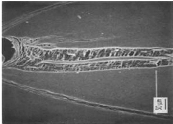
Fig. 5.22 Cold drawn behavior of a thermoplastic polymer up to failure
