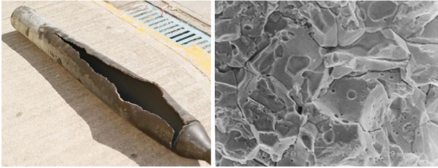
Fig. 8.11 Macroscopic (left) and microscopic (right) appearance of a typical creep fracture
